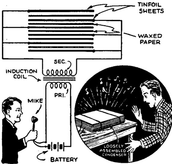
to excite the condenser may be a telephone type coil, an old shocking coil or a small spark coil; even an ignition coil may be used in a pinch. An ordinary microphone is connected in series with a battery of a few dry cells and the primary winding of the induction coil. The condenser really forms an electrostatic loud-speaker, and as the fluctuating electric charges caused by speaking into the microphone reach the condenser leaves, they vibrate in unison with the voice.
