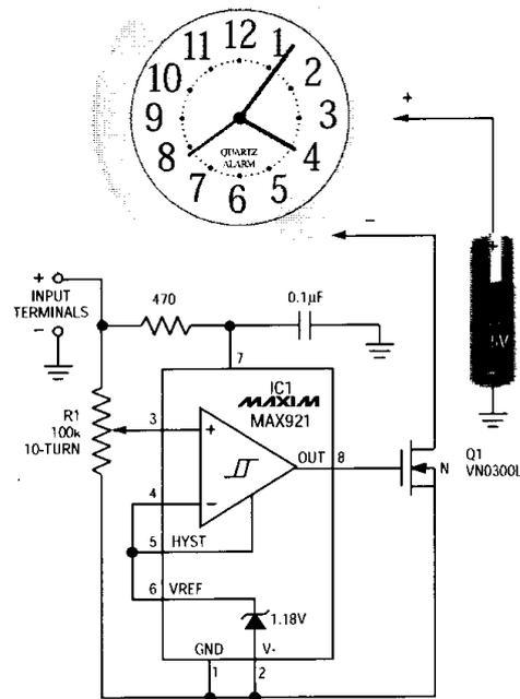
Figure 1. This inexpensive clock tracks the operating time for a battery-powered portable system. When the battery voltage (or a selected output) drops below the discharge threshold set by R1, the stopped clock retains the elapsed operating time.
