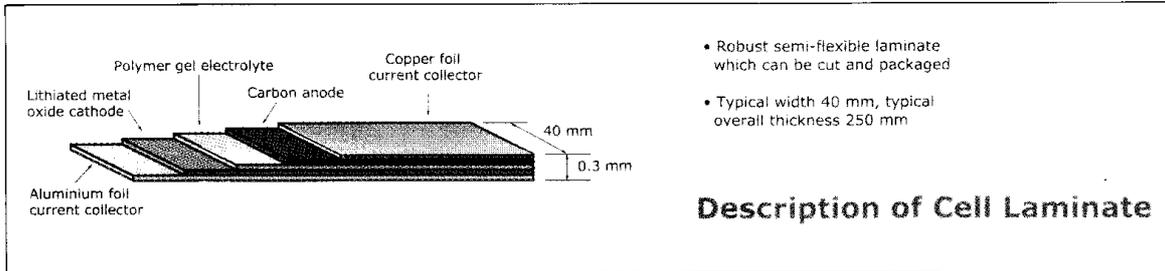
*Laminated cell fabrication via a continuous process. The polymer gel electrolyte: (i) holds the laminate together; (ii) separates the electrodes; and (iii) provides high lithium ion conduction.*
