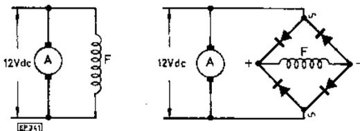
HERE is an unusual and interesting application for a bridge rectifier. A colleague of mine was building a device which is powered by a shunt wound d.c. motor (actually a discarded windscreen wiper motor) and he required the motor to be reversible. Because supply reversal causes reversal of the current in both the armature A and the field F, the motor remains stubbornly unidirectional. Fitting a switch on the motor to reverse only the field current was not possible as the motor
